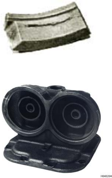
Figure 3-59. Magnetic Particle Indications of Defects in Castings
