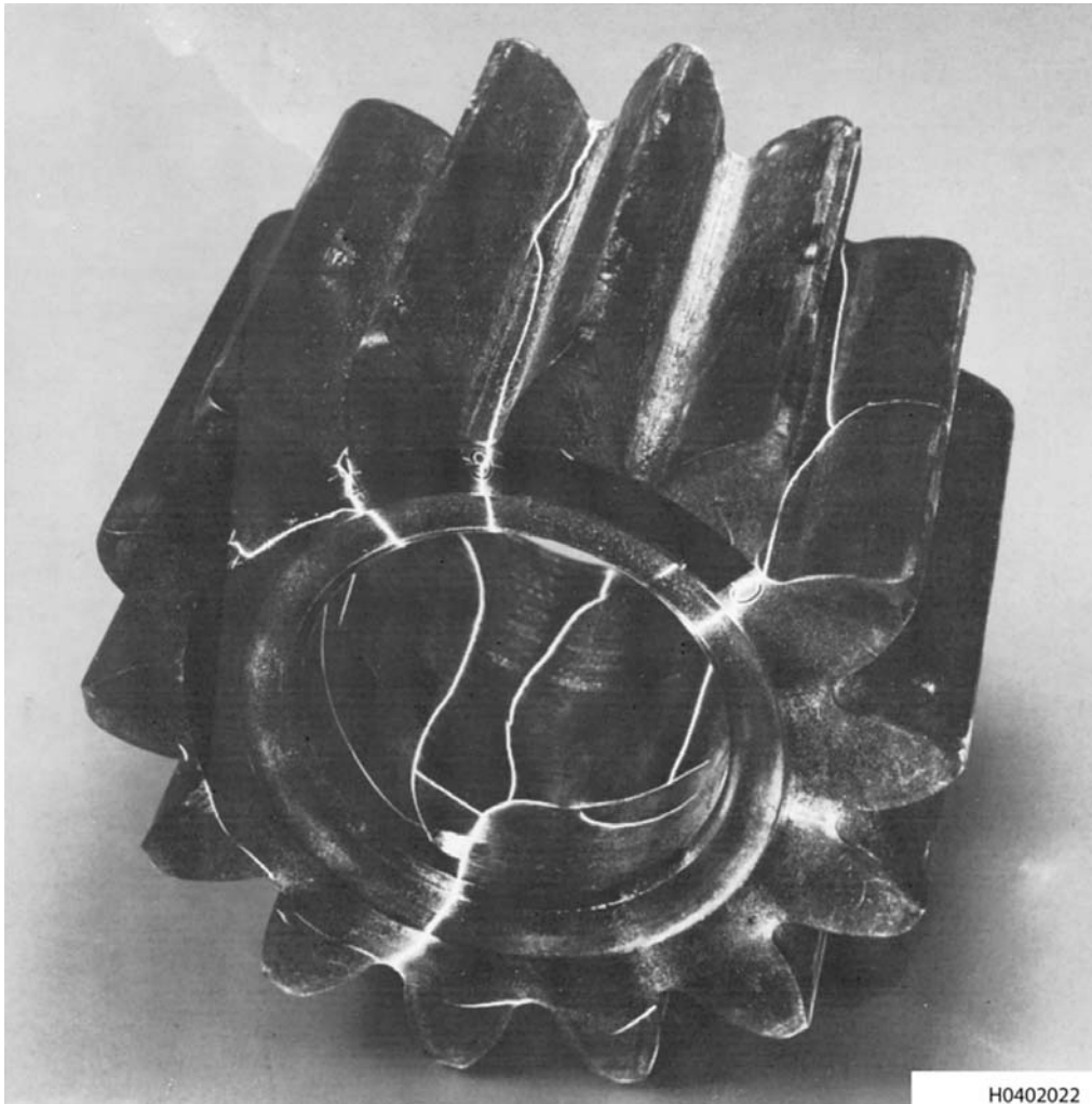
Figure 3-41. Typical Magnetic Particle Indications of Cracks
